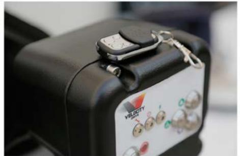
Our innovative remote control device, allows you to raise and lower your landing legs wirelessly from inside the drivers cab.
